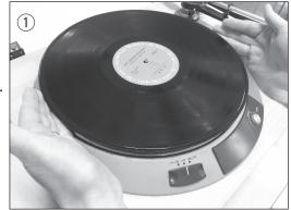
② Insert the suction collar in the center spindle and press the switch on the suction box. Suction operation ends when operation lamp goes out. (Adsorption is done in about 30 sec.) In case adsorption is not done well enough due to the warpage of a record disc, try to press the switch again or set the suction adapter to have it fully adsorbed. (The surface being fluffy when press a record disc means adsorption has not correctly been done.)
